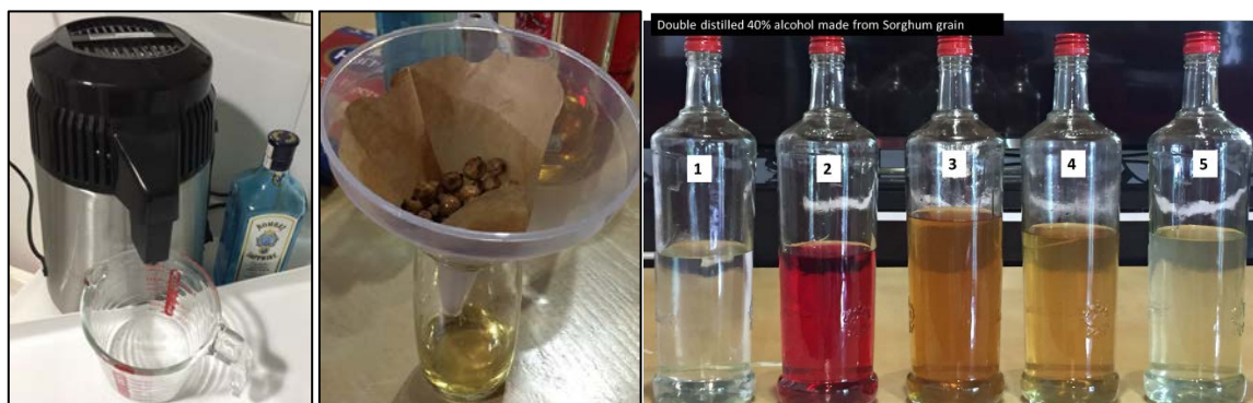
Figure 12. Left: Air Still in operation producing 50-60% clear alcohol after double distilling. Centre: Flavour infusion achieved by soaking and then filtering locally sourced (CI) and imported ingredients into 50ml of 60% alcohol. Right: The finished product 1) no infusion; 2) Juniper berries, dragon fruit, dried lime peel, Kaffir lime leaves; 3) Juniper berries, soursop (custard apple), dried lime peel, dried orange peel; 4) Juniper berries, lemon grass, coriander seed, star anise, cinnamon; 5) Juniper berries, Japanese cherries.
